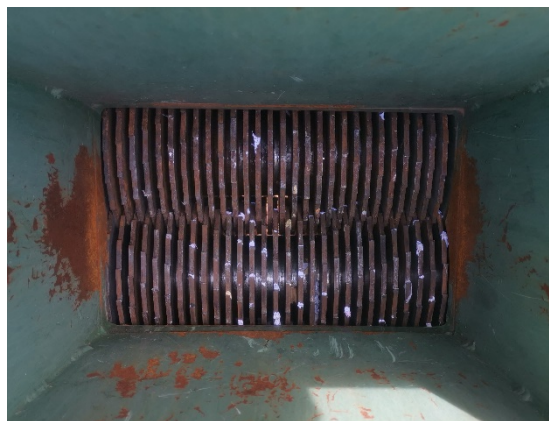
Figure 2: Shredder cutting elements/blades
